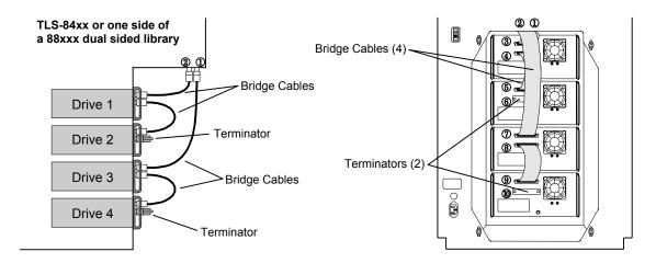
Figure 4-2 TLS-54xx, 58xxx, 64xx, 68xxx, 84xx and 88xxx Drive Cabling Diagram
